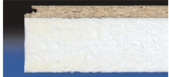
A high performance, rigid expanded polystyrene insulation bonded to tongue and groove chipboard with a thermal conductivity of 0-029 – 0-030.
